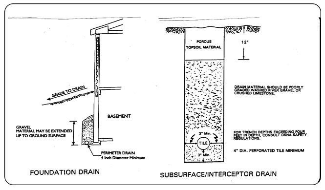
It is a good practice to install subsurface drains, which are at least 4 inches in diameter and are surrounded with gravel or sand. If at all possible, the drain pipe shoud have 2 feet of cover.
