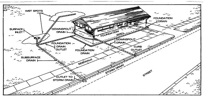
Control of external water around and beneath a house is essential. Mildew, wood destroying fungi and wet insulation will result when surface water floods or saturates the ground around and under a house. *Techniques that will reduce external water problems are:*
