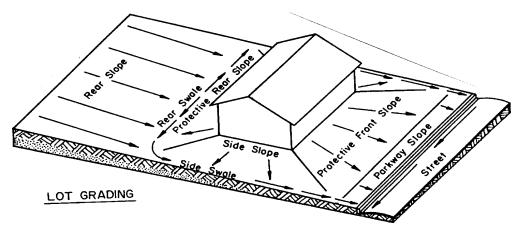
*Figure 1* above illustrates the most common drainage problem of a sloping lot. The uphill side of the house must have a drainage waterway (swale) to direct the water around the house. This drainage swale should be at least 10 feet from the house and sloped to convey accumulated water away from the dwelling efficiently, and into a proper outlet.
