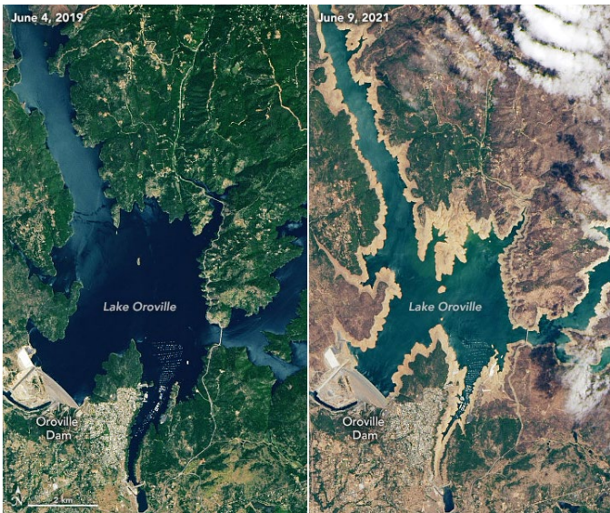
Satellite images of Lake Oroville, a reservoir in northern California. Left: At capacity (highest level), June 2019. Right: At a much lower water level due to drought, June 2021. In August 2021, the Edward Hyatt Power Plant, a hydroelectric plant on Lake Oroville, was shut down because water levels were too low. Source: USGS (public domain) .
