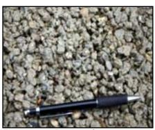
Figure 2.11.6 Pervious Concrete
