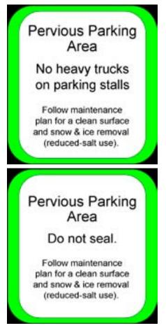
Figure 2.11.13 Examples of signage that might be used to protect pervious pavements.
