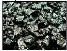
Figure 2.11.5 Porous Asphalt
